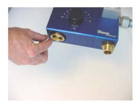
2. Remove nozzle (26) with spacer sleeve (27) and twist (28)
