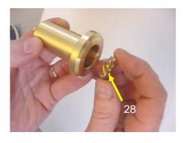
5. Carefully insert the twist (28) into the nozzle (26). Make sure it is <u>not jammed</u>.
