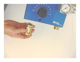
6. Install the completed nozzle (26+28), and the spacer sleeve (27) into Jetmix.
